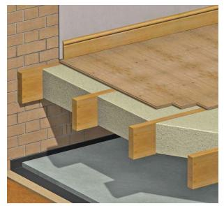
Figure 03: insulating / refurbishing ground floors
