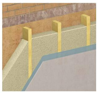
Figure 01: insulating timber frame walls
