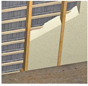
Figure 06: insulating / refurbishing pitched roofs
