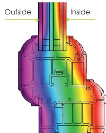
The cross section to the right shows how Liniar's multi-chambered profile prevents the transfer of heat from the inside to the outside.
