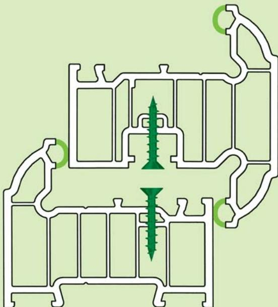
The **eco energy plus** window system uses its multiple chambers to lock in the heat, and high performing bubble gasket seals to ensure there are no gaps for heat to escape.
