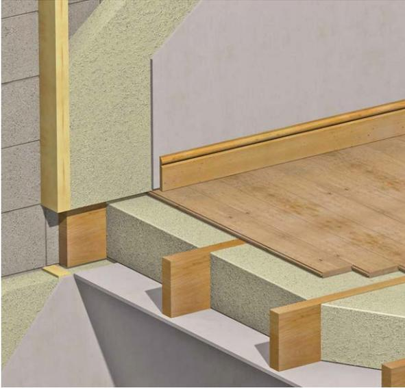
Figure 04: insulating / refurbishing walls and intermediate floors
