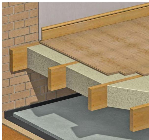
Figure 03: insulating / refurbishing ground floors
