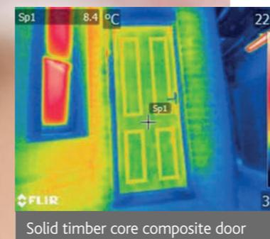
Doors were tested at the University of Salford's Energy House. This represents a typical Salford 1919 terraced house and its construction represents 21% of the UK's current housing stock. The house has been reconstructed in a fully environmentally controllable chamber, in which climatic conditions can be maintained, varied, repeated and patterns monitored. For the test, the inside temperature of the Energy House was 25°C with an exterior temperature of 5°C.
